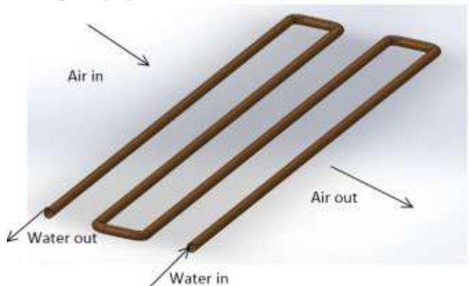
Fig 2. Simulated row of heat exchanger
