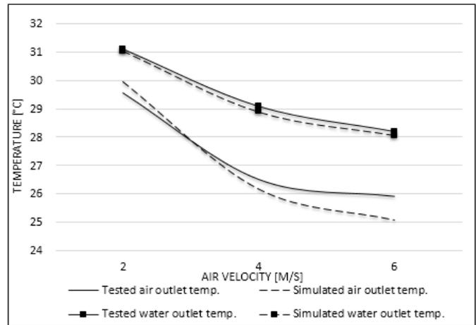
Fig 3. Simulated vs. tested: outlet temperatures 21 – 23 °C – 25 l/min
