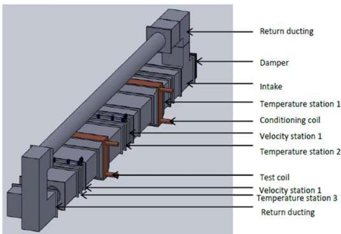
Fig 1 Layout of test bench [9].
