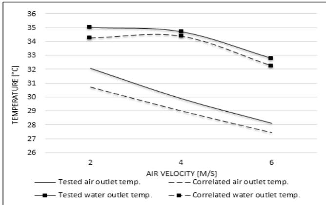
Fig 9. Correlated vs. tested: outlet temperatures 21 – 23 °C – 50 l/min
