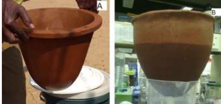
Fig 1: The ceramic water filters from (A) Mukondeni, Limpopo province of South Africa and (B) Sese, Masvingo province of Zimbabwe
