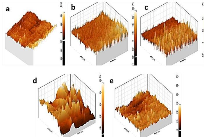
Fig. 4 Topography of Ti-6Al-4V after wet etching. SPM micrographs of Ti-6Al-4V alloy after a) polishing, etching with b) strong Kroll, c) weak Kroll, d) sulfuric acid and e)alkali etching for 60 min
