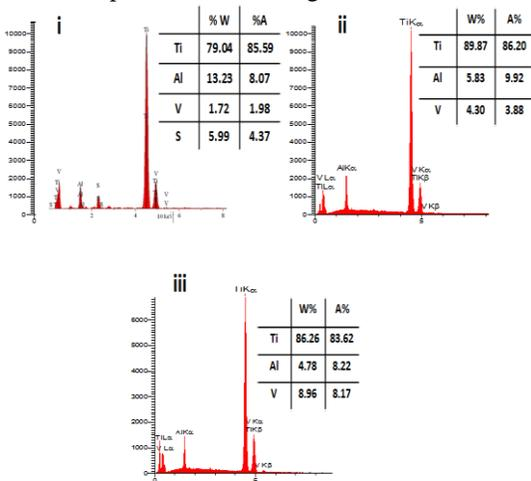
Fig.3 EDX analysis of point (i) showed in Fig.1.ii) black zone pointed as (ii) and iii) matrix pointed as (iii) in Fig.2.
