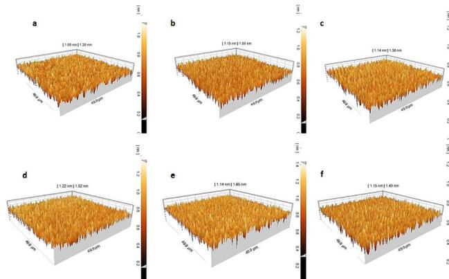
Fig. 5 Effect of etching time on the topography of modified Ti-6Al-4V alloy. SPM micrographs of Ti-6Al-4V alloy after etching with a-c) weak Kroll and d-f) strong Kroll after 15-60 and 120 min, respectively.
