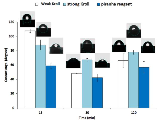
Fig. 7 Contact angel of pure water on modified Ti-6Al-4V alloy.
