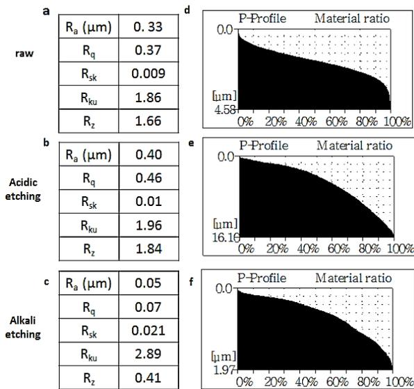
Fig. 6 Roughness results of a) polished and modified Ti-6Al-4V alloy with b) Strong Kroll, c) piranha for 60 min.
