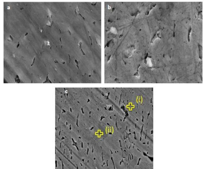
Fig.2 Alkali etching of Ti-6Al-4V alloy. Selective etching of  $\beta$ -phase. FESEM images of Ti-6Al-4V alloy etched by piranha solution for a) 15, b) 30 and c) 120 min. Scale bars are 2  $\mu m$ .
