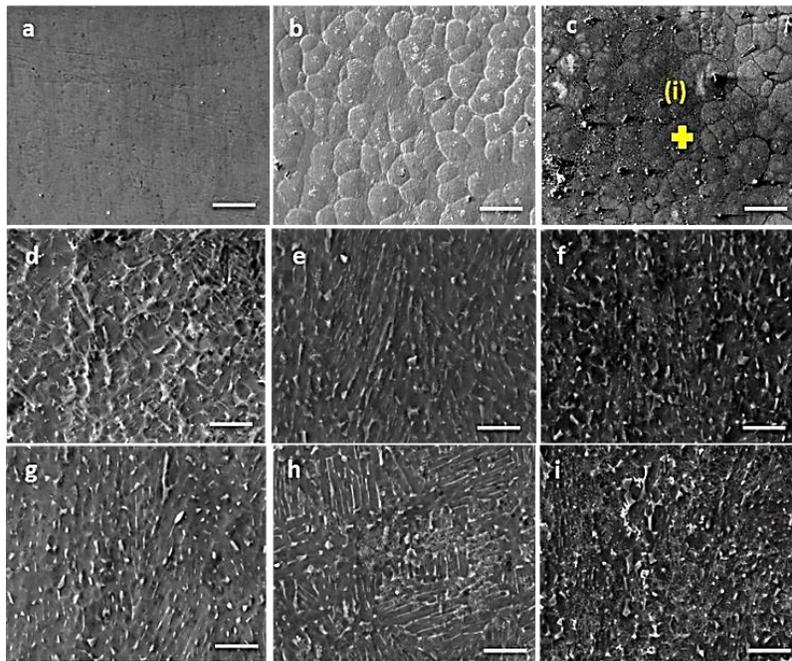
Fig.1 Acid etching of Ti-6Al-4V alloy. FESEM micrographs of Ti-6Al-4V alloy after exposing to single acid a-c) ( $H_2SO_4$ ) and double acid-etching d-f) weak Kroll, g-i) strong Kroll for 15, 30 and 120 min, respectively. Scale bars are 50  $\mu m$ .
