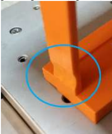
Fig. 10. Introduced damaged on one of the columns
