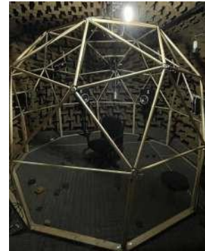
Fig. 1. The physical implementation of the multichannel loudspeaker array.
