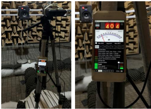
Fig. 4 Mobile phone and SPLnFFT application in calibration tests
