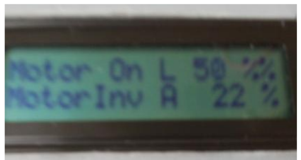
Figure 14: Display of the microcontroller showing the percentage of pulse width (L) and the delay/advance (pulse position A).
