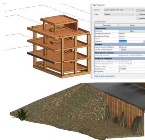
Fig. 5. Formwork of the structural elements and berlin wall to support the excavation work.
