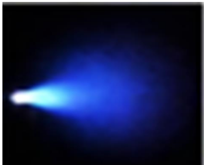
Fig. 1 Plasma image formed by ablated ZnO particles
