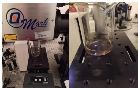
Fig. 2. CTS nanoparticle production in ethanol medium using Q-Mark micromachining unit
